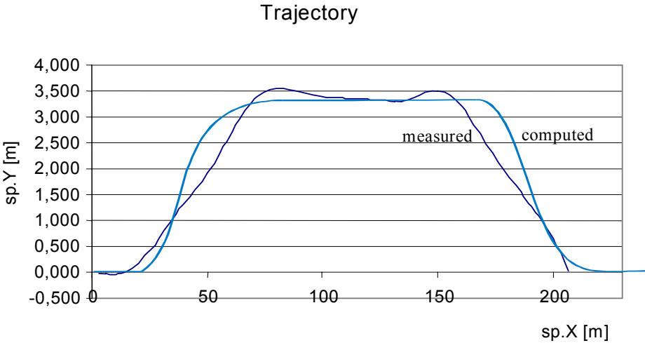
Fig. 14 Simulation-experiment comparison: computed and measured data, 50 km/h
