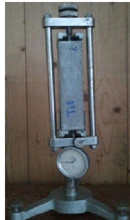
Fig. 2. Device to assess the dry shrinkage according to SREN 12617-4
