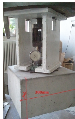
Fig.4. Developed tension test rig for confined tests
