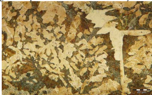
Fig. 6. Sample microstructure microalloyed with Mn
