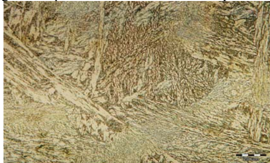
Fig. 5. Sample microstructure microalloyed with B
