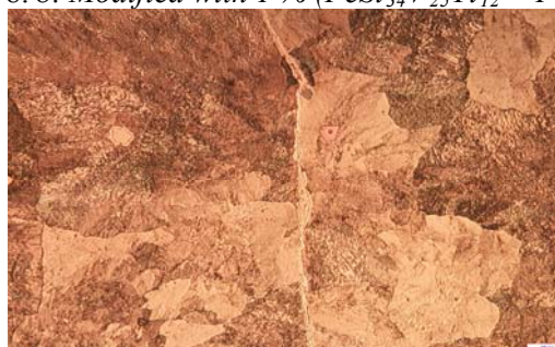
Fig. 8. b. Modified with 1 % ( FeSi_{34}V_{25}Ti_{12} + FeB_{15} )
