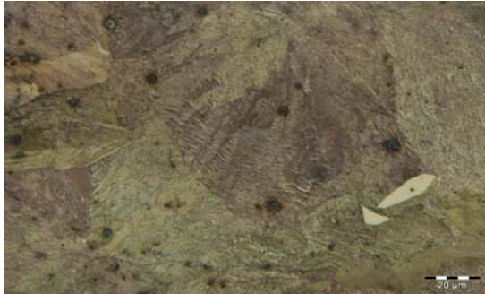
Fig. 3. Sample microstructure microalloyed with Cu
