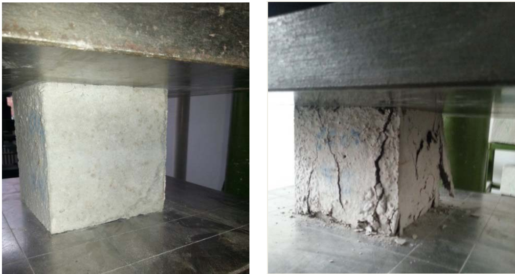
Fig. 7. Determination test for compressive strength with 300tf UTM (300tf Universal Testing Machine)
