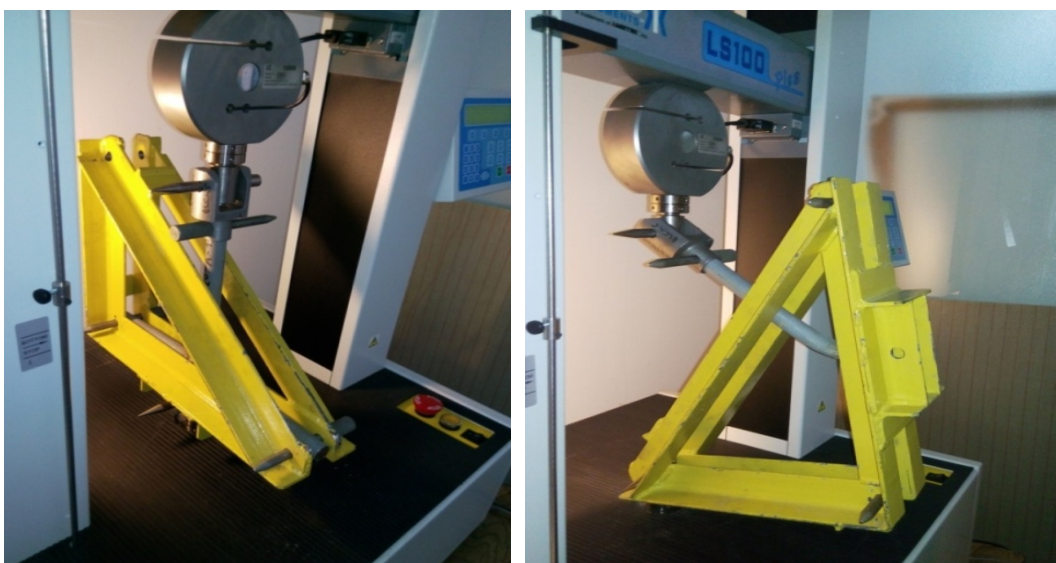
Fig. 9. The testing interface installed on the LS100Plus testing machine (AXL/ IPB)
