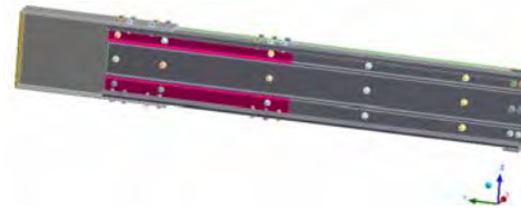
Fig. 12. The joint assembly of thin walled steel profiles KB for the KB450-3.5 beam
