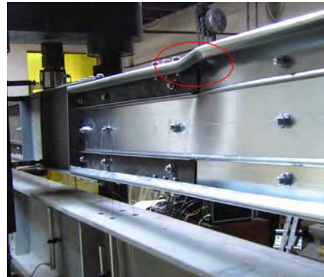
Fig. 7. The local buckling of the KB element for the R-KB450-3.5 beam
