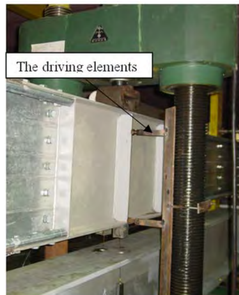
Fig. 4. The driving elements mounted to prevent the lateral buckling.
