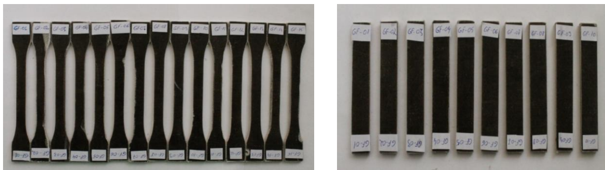
a) b) Figure 1: Specimens cut on the weft direction of the flax woven fabric: a) tensile specimen; b) specimens for flexural test
