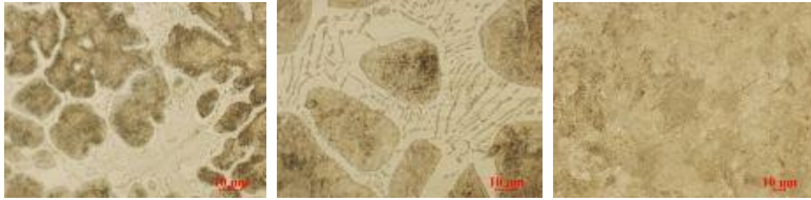
Figure 9: Structure of steel mould cast ZnAl 22 alloy: (a) sample a - 0 - in cast state; (b.) sample a - 2 - DIL – partial melting, and (c) sample a - 1 - 1-DIL, no melting
