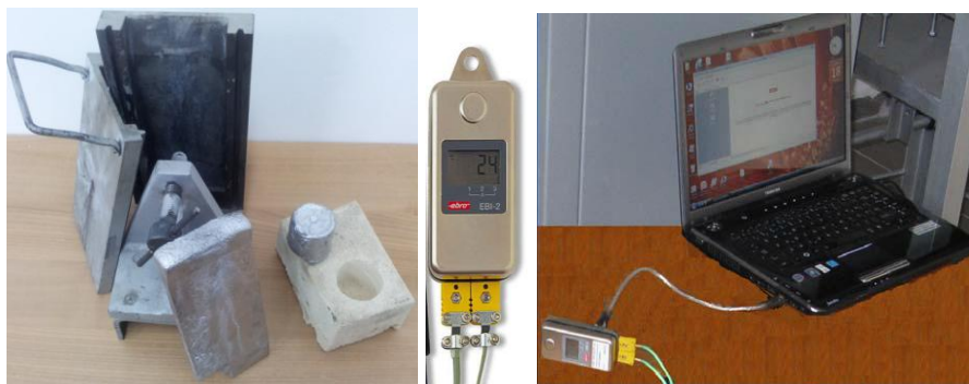
Figure 2: Casting moulds and assembly for cooling curve recording
