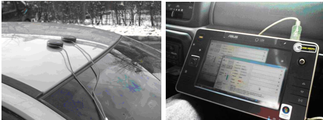
Fig. 6 – Example of a DS-5 system installed on a vehicle (version with 2 receivers)
