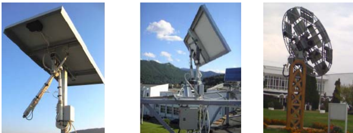
Figure 4. Tracking systems designed and implemented at Transilvania University of Braşov: a) pseudo-equatorial [3], b) azimuthal [15], c) pseudo-equatorial platform [5]
