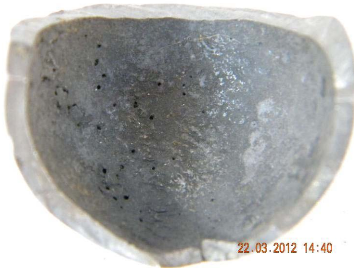
Figure 4. Defect of the ball made by the breaking of the outer layer
