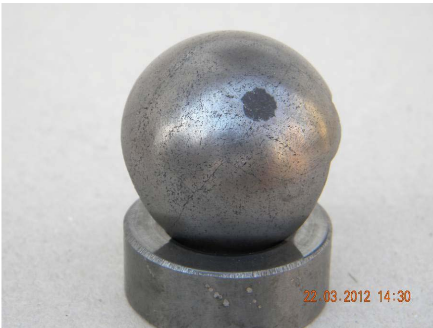
Figure 3. The valve (ball and seat) of piston pump for oil extraction
