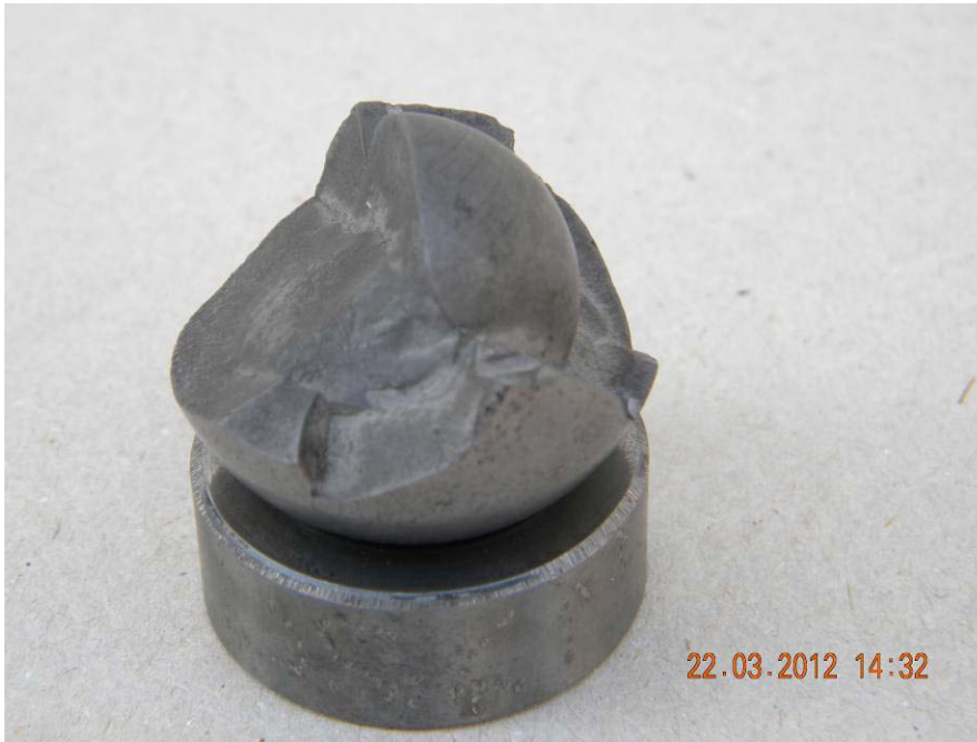
Figure 5. Defect of the ball made by the breaking of the outer layer and a piece of initial ball
