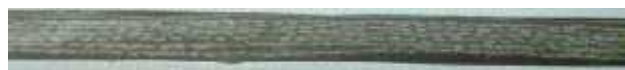
Figure. 5. Specimen viewed from the side with the 6 layers of fiberglass fabric 280\text{g/m}^2 thickness , [1]
