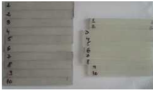
Figure. 8. Sandwich structure consists of two test-piece fiberglass reinforced with ABS and nylon 6/10
