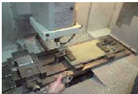
Figure. 4. Cutting specimens in 100mm length, width 10mm and 5mm thick.
