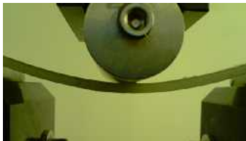
Figure .10. Bend testing a fiberglass specimen
