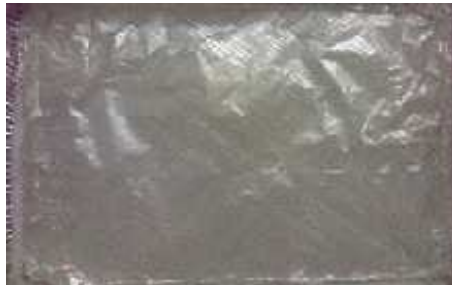
Figure. 3. Composite board structure consisting of epoxy resin with hardener and 2 layers of fabric reinforced nylon 6 / 10
