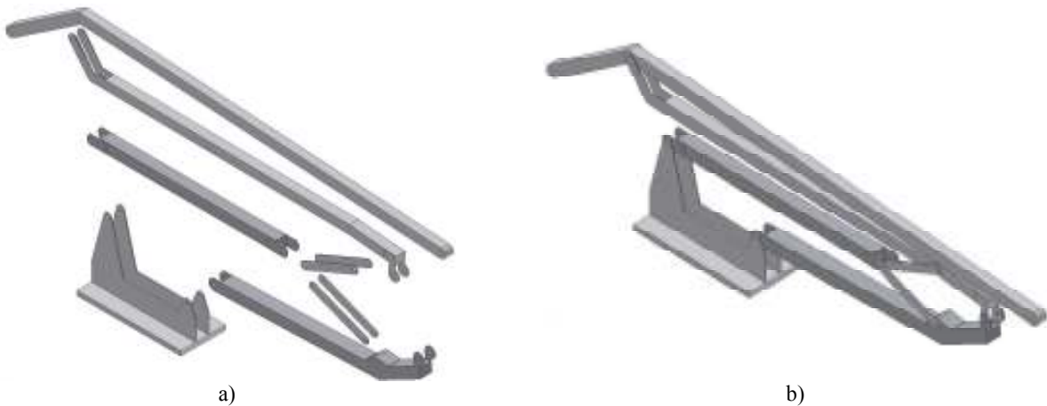
Figure 6 a) Built parts of the mechanism, placed in position to apply the geometric constraints; b) applied constraints between kinematic elements;
