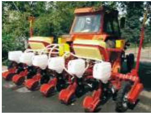
Fig. 1: Equipment for sowing and fertilizing hoeing plants crops provided with sections of disk plows and equipment with distribution of insecticides in granular form
