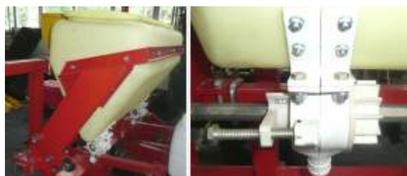
Fig. 5: Hope fertilizer provided with fertilizer distributors type with grooved drum
